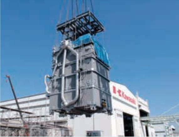
The world's largest off-shore boiler, designed for the Prelude FLNG, has been delivered to the site. The boiler is a compact, modular unit that can be transported by sea. It is designed to operate at a maximum steam flow of 1,200 t/h.
